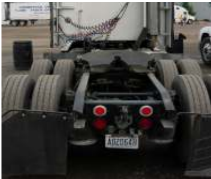
Truck frame, wheels, and fifth wheel
