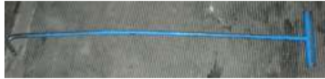
Tool used to “pop” the trailer release (32” long)
