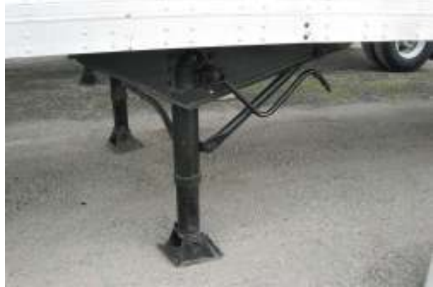
Trailer landing gear (approx 10 lbs. to crank once trailer is attached to truck)
