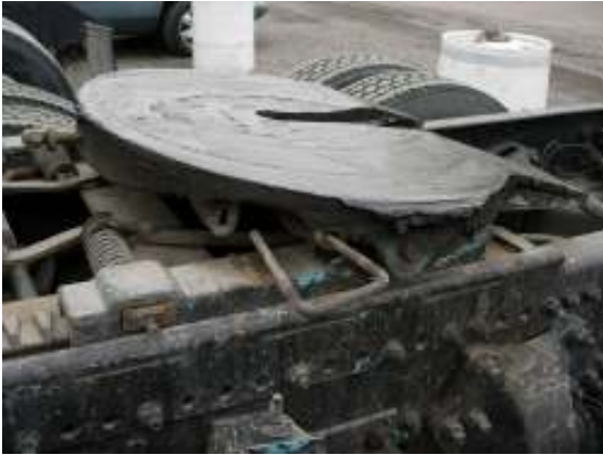
Fifth wheel (with trailer release handle)
