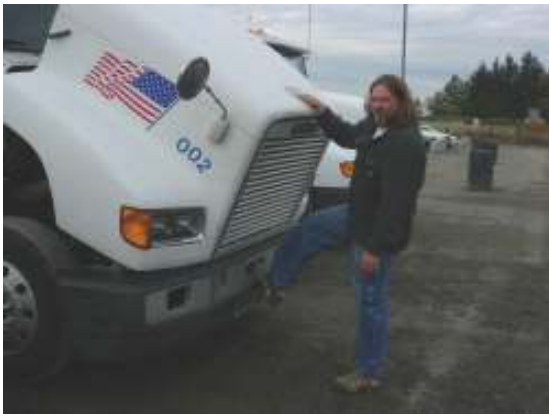
Truck hood (Fiberglass – 60 lbs of force to open)
